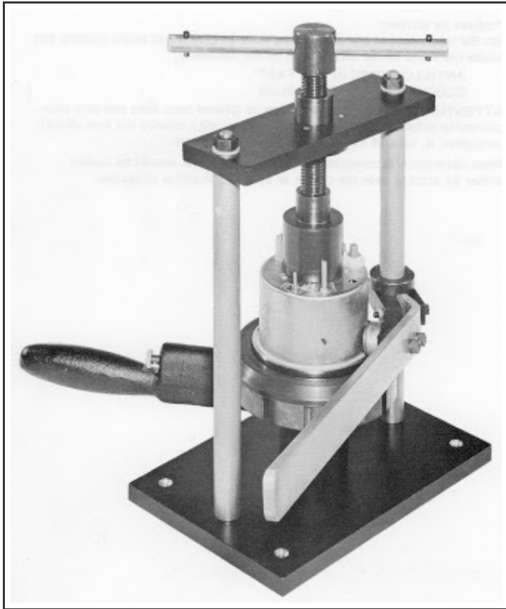
A Smiths bezel rolling on tool to illustrate a re rolling on operation...
