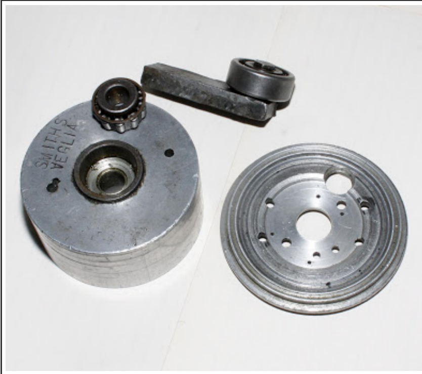
Tooling you can make...a ballrace attached to a bar to do the rolling on...an aluminium plate with a suitable "V" of the correct diameter to lock the assembly while the bezel is rolled over. The large block has holes drilled in it to fit over the back of the speedo and allow you to push against the seals/glass for a water-tight seal as you
